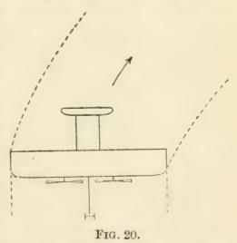
to "bank," or tilt, the machine inwards, so as to correct this tendency. By the tilting of the surfaces the lift is naturally decreased, especially with
